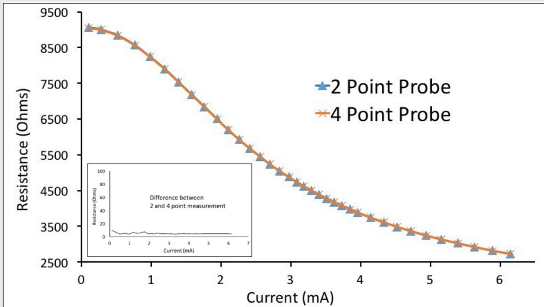
**Figure 3:** A comparison between 2 and 4-point probe measurements on a MEMS heating device with a ceramic heating membrane. The Electrical Current vs Resistance measurements are identical. The inset graph shows the magnitude of the difference between 2 and 4-point probe measurements. This corresponds to a maximum error of less than 0.2%
