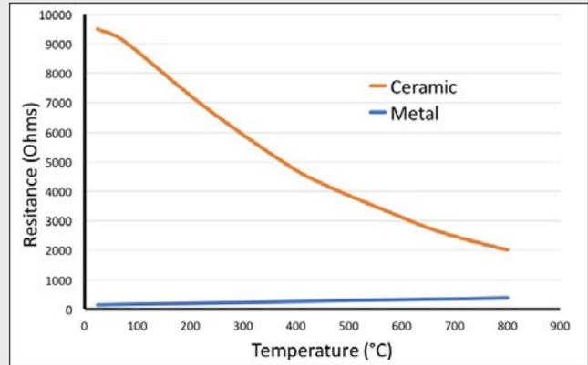
**Figure 2:** The change in resistance versus temperature. Comparison between metal and ceramic.
