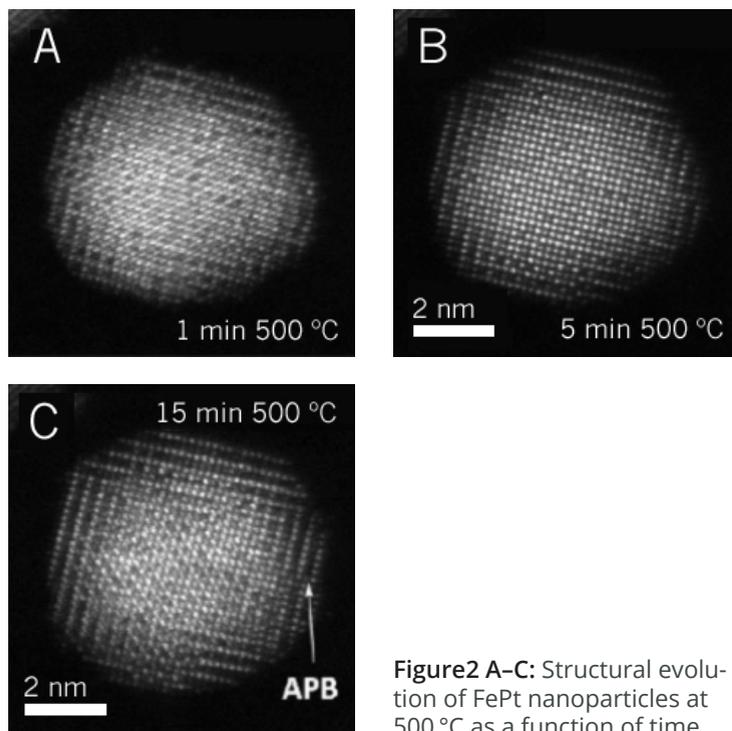
Figure 2 A–C: Structural evolution of FePt nanoparticles at 500 °C as a function of time
