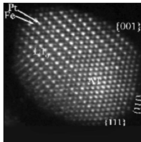
Figure 1: FePt nanoparticles
