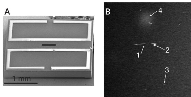
An SEM image of the GapSet E-chip used to form the microfluidic channel is shown in Figure A. Figure B shows a STEM image of nanoparticle flow. A series of streaks is visible at arrow 1, which presumably are due to a single gold nanoparticle moving to the left.
